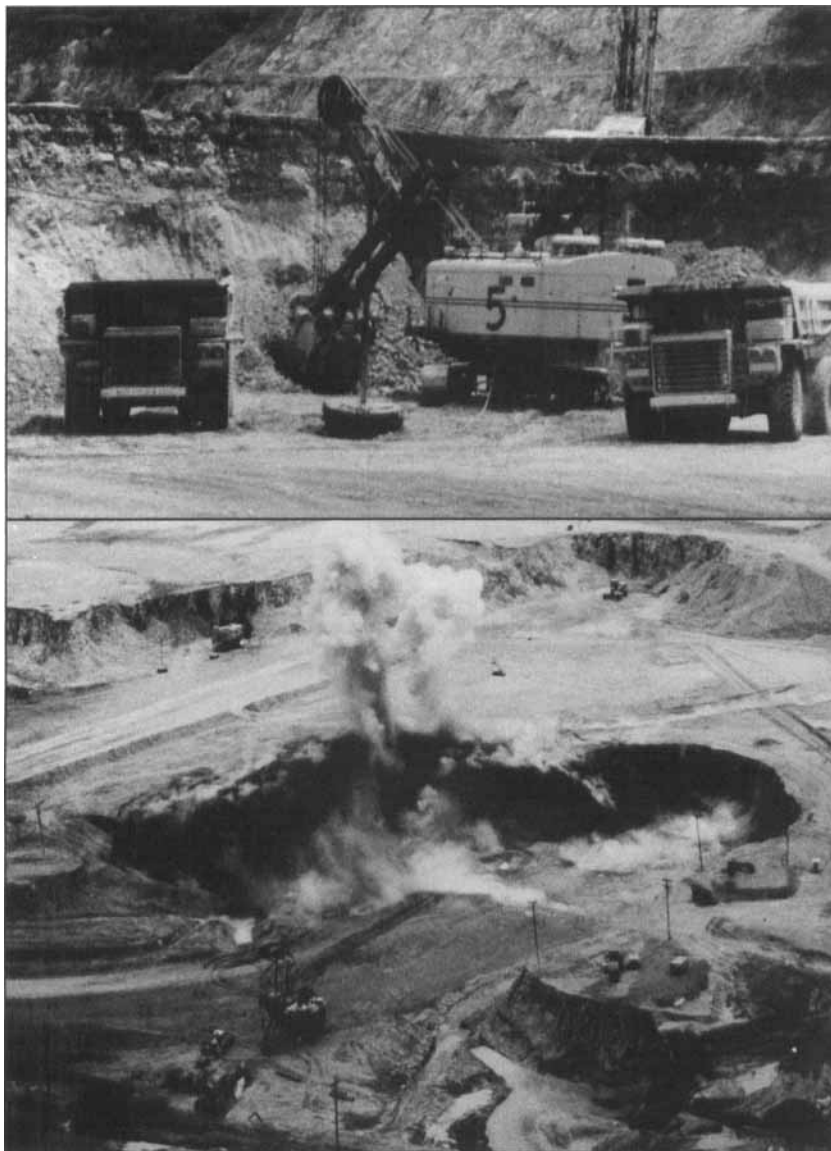
Above: Mining at Panguna: Euclid R190 haul trucks and P & H 2800XPA electric shovel which, with each scoop can take about 25 tonnes of ore.
