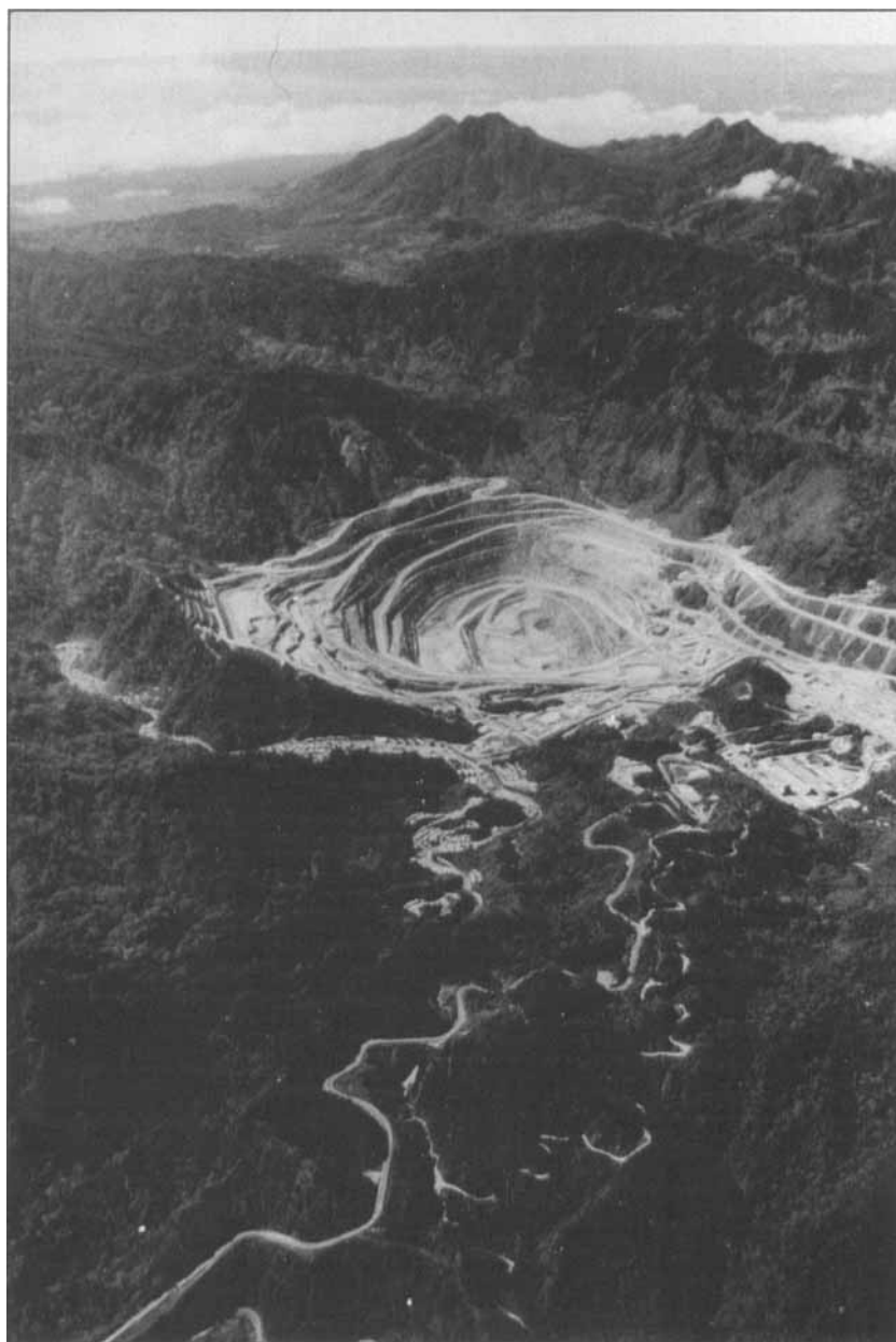
Aerial view of the Panguna mine taken in 1978. Mine access road in the foreground, crushing and flotation facilities at right.
